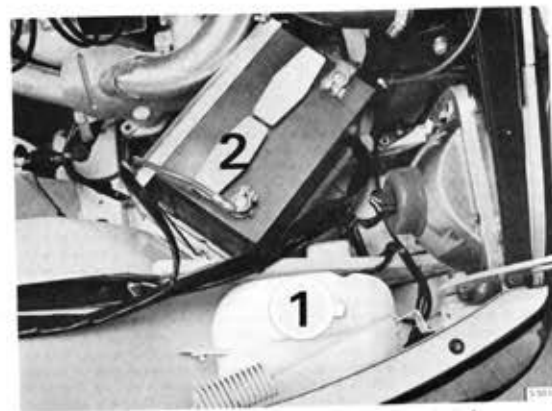
Location of washer fluid container 1. Washer fluid container. 2. Battery
