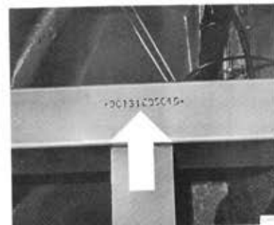
Chassis number punched in car body, 4- and 5-door models (under back seat cushion)
