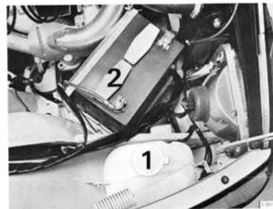
Washer fluid and battery
