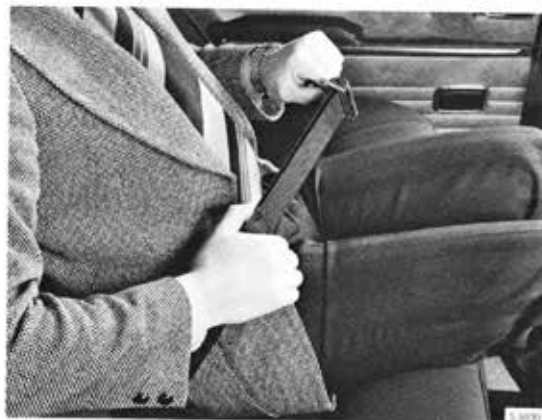
Lengthening the middle rear-seat
