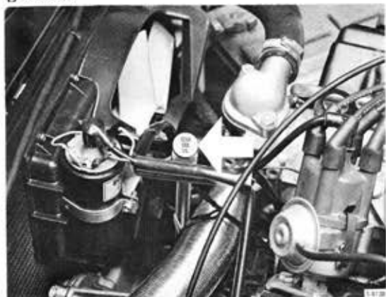
Location of dipstick, automatic transmission
