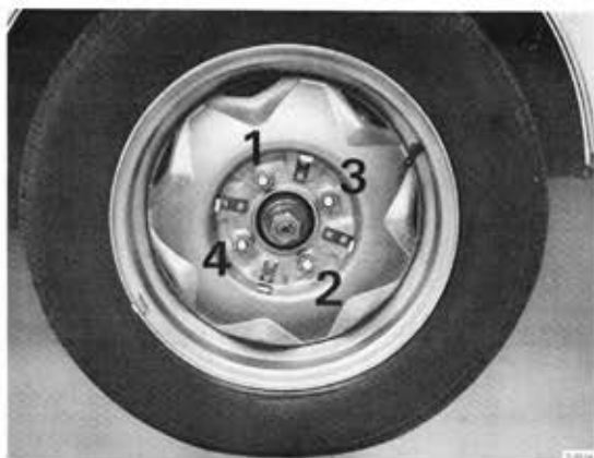
Order of tightening wheel nuts
